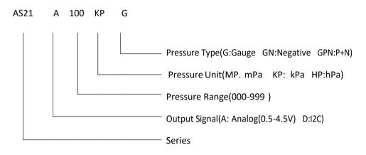
Note: 5Vdc as default power voltage, add 33(or 30) behind model signify 3.3V(or 3.0V) power supply, e.g. AS21040KPG33(or AS21040KPG30).
