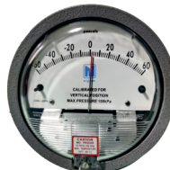
100mm Dial, Back Mounting, 1/8" NPT-2 Nos PC, Available in mmWC, Pa, WC
